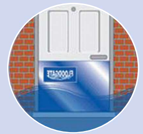
Step 3: Floodgate in place
